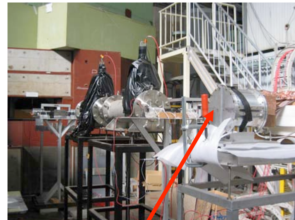
Carleton TPC in the beam outside the magnet
